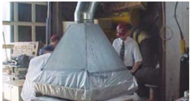
IFD air leakage testing at CSIRO.
